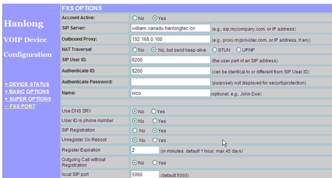
The screenshot shows the 'FXS OPTIONS' configuration page. On the left is a navigation menu with 'Hanlong VOIP Device Configuration' and links for '+ DEVICE STATUS', '+ BASIC OPTIONS', '+ SUPER OPTIONS', and '- FXS PORT'. The main content area contains the following fields:
